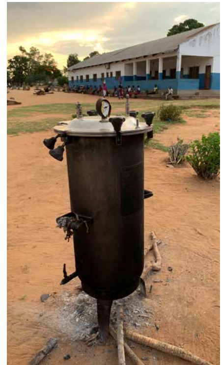
▲ Charred bits of firewood below the defective steriliser, evidence of the health workers makeshift attempts to heat the water in the device. bg
